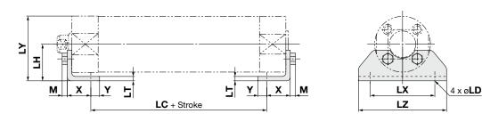
Foot bracket material: Stainless steel Mounting bolt material: Stainless steel
