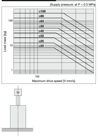
• A case where the center of gravity of the load rests 50 mm from the rod end.
