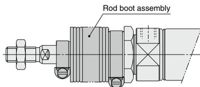
\* Replaceable with the rod boot assembly
