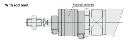
\* Replaceable with the rod boot assembly For details on replacement part numbers, refer to page 243.
