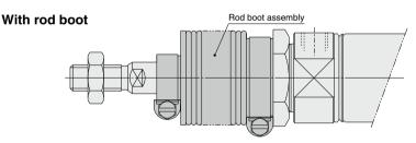
\* Replaceable with the rod boot assembly For details on replacement part numbers, refer to page 243.
