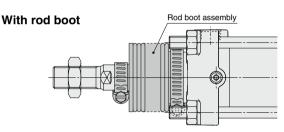
\* Replaceable with the rod boot assembly For details on replacement part numbers, refer to page 248. (CA2-Z only)
