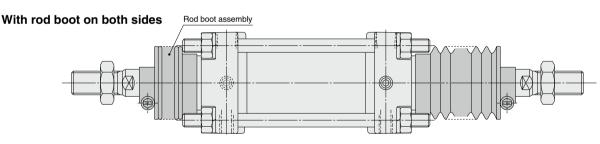
Replaceable with the rod boot assembly
