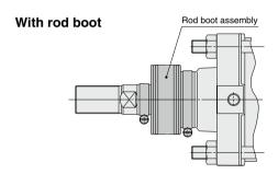
\* Replaceable with the rod boot assembly For details on replacement part numbers, refer to page 251.
