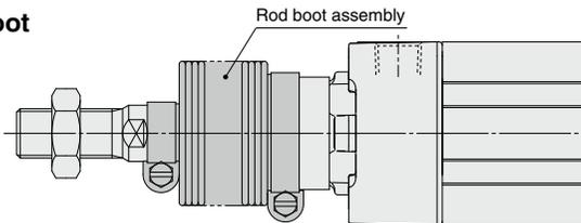
\* Replaceable with the rod boot assembly
