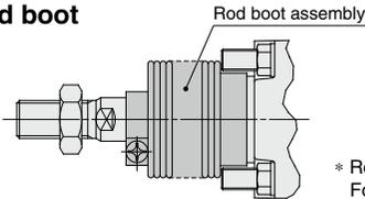
\* Replaceable with the rod boot assembly
